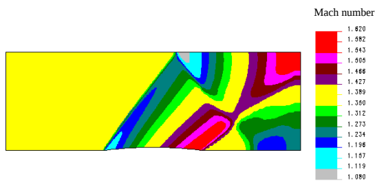
Mach number contour for Mach 1.4 flow past a 4% circular bump. 2D solution.
